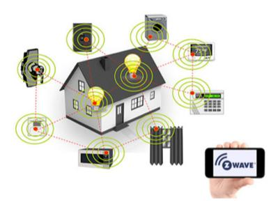
Designed for devices built on the Z-Wave 700 platform, the v2 certification includes SmartStart, a feature allowing hubs to recognise any SmartStart-enabled accessory with a quick app scan of a QR code. Through SmartStart the device information is already set up in the hub, and pairing is complete prior to the consumer adding the product. Thus, the product setup process is both shorter and simpler.
