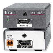
Used at the destination end of a long cable run, the HD 4K 101 Plus actively equalises poor or marginal sources signals, reduces jitter and skew, and adds output pre-emphasis to reliably extended HDMI signals. Extron says it can handle longer distances of up to 22 and 10m for 4K@30Hz and 4K@60Hz signals respectively if paired with an HDMI Pro Series cable.
