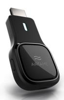
As presented at CES 2014 the Airtame package consists of the dongle and PC (Mac, Windows, Linux) app. Users simply plug the dongle in a display's HDMI port, and the app handles either mirroring (complete with audio) or display extension.
