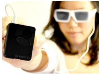
The ActivEyes system comes in 2 parts; the glasses (weighing only 29g and usable for passive 3D) and a separate integrated electronics-carrying mini "box" for active shutter TV, which the user connects to the glasses.
