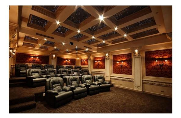
Designed to add the beauty of a night sky to any room with a drop-in ceiling, the tiles are a more affordable alternative to the original, custom-only StarField Ceiling Panels from the company. Fabric-wrapped fibreglass panels improve sound quality in any space, taming reverberation and ambient noise, and connect to main lighting control systems via RS232 adapter.
