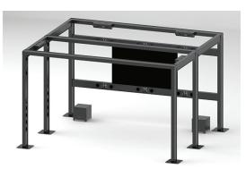
The theatre consists of a built-to-size aluminium structure installers assemble onsite. It houses all required loudspeaker components for any surround format, and is compatible with an array of subwoofer options depending on the decor and acoustic requirements of the space in question.
