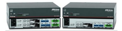
The individually bridgeable channel pairs of the XPA U 1004 SB can deliver two 100 watt channels into low impedance systems or one 200 watt channel into low or high impedance systems, while the XPA U 2002 SB delivers 200 watts and 400 watts respectively. A rotary switch on the rear panel of the amplifier makes it easy to select the desired output mode.
