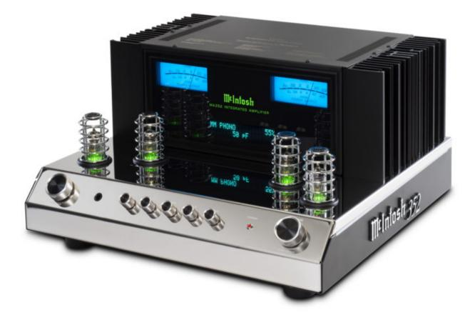
The all-analog design has a vacuum tube preamplifier section powered by a pair of 12AX7A and a pair of 12AT7 vacuum tubes. The output stage is a direct coupled solid-state amplifier outputting 200W per channel into 8-ohm speakers or 320W per channel into 4-ohm speakers, making double the output of the previous McIntosh integrated amplifier, the MA252. Dual scale blue Watt speakers give an accurate power output readout for both speaker impedances.
