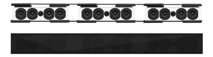
Featuring an 8-ohm impedance, the soundbar incorporates three speaker enclosures with six 3-inch ultra-long throw polypropylene subwoofers with NBR surround sound and a 0.75-inch synthetic soft dome tweeter. It is 9.6cm deep and 15.5cm tall, and is designed for applications demanding a width of 1.4m or longer.
