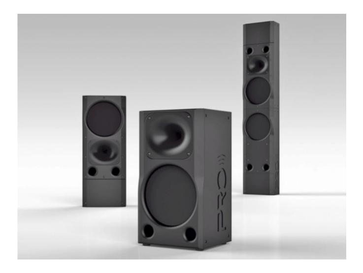
The loudspeakers replace 3 existing PRO models, namely the SCRS-12s, SCRS-12ai and the SCRS-212ai. Both S and SR series employ a 1.7-inch Ultra-Purity high-frequency compression driver mounted on an elliptical wide coverage horn. Designed for placement behind an acoustically-transparent screen, the S-12sm and SR-12ai feature a 12-inch 1400W long-throw woofer with a 4-inch voice coil.
