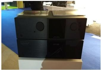
The Altitude16 renders up to 16 discrete channels of information, and features Dolby Atmos, Auro-3D and DTS:X immersive audio decoders. It natively processes high-resolution 24/96 audio, and Trinnov claims it has no limit in terms of subwoofer outputs. Also included is support for 4-way active crossovers.
