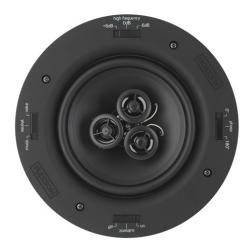
The 65X3 promises flexible installation, since it is mountable in shallow ceiling voids with 50mm minimum space. It is also moisture-proof, allowing use in kitchen or bathrooms without complication. Room tuning options include a high frequency boost/cut 6dB switch and a bass attenuation switch for level control in case the speaker is located in a large void.
