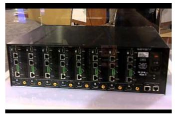
The SmartLink switch is available in 3 versions, each with 8 HDMI inputs and 8 S/PDIF audio-only outputs and a choice of 4, 6 or 8 HDBase T 5Play or HDMI outputs-- in other words enough control ports for easy audio and video source management.
