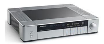
Inputs include 1 MMHR (Meridian Multichannel High Resolution) port designed to accept audio from an own HDMI switcher, 2 SpeakerLink inputs, 6 S/PDIF inputs, 2 Toslink ports and 8 analog phono (RCA) ports.
