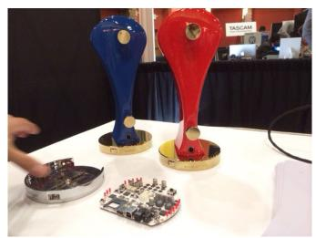
Standing 30cm tall with a design complete with metal knobs for secure cable winding, the Gemini docks are controllable via onscreen PC interface and decode high-resolution DXD, DSD and double-rate DSD audio at sampling rates from 44.1kHz to 384kHz.
