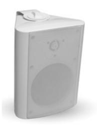
The OL-70v is, as the name implies, rated at 70V but is switchable to 8 ohms impedance if required. Taps are 2.5W-25W selectable, with a large ABS cabinet housing a 6.5-inch polypropylene MF/LF driver and a 1-inch silk dome tweeter.
