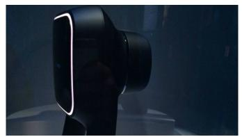
Being an early prototype, the unnamed device lacks built-in audio, requiring the addition of external headphones. What it does have is a pair of 2560x1440 5.5-inch LCD displays (for total 5k resolution), a lens assembly featuring 3 glass elements per eye and 120-degree field of view, making it superior to the likes of the Oculus Rift or Samsung Gear VR.
